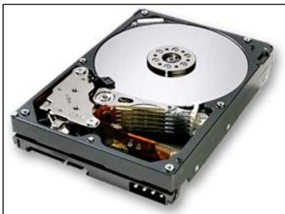
The **hard drive** on your computer is where the software is installed, and it's also where your documents and other files are stored. The hard drive is long-term storage, which means the data is still saved even if you turn the computer off or unplug it.
