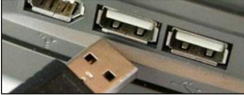
**Universal Serial Bus (USB)** is by far the most common port that are used with computers. As the name suggest Universal, this has become the most common standard that most peripherals use today. A mouse, keyboard, flash drives, and even smartphones to upload your pictures.
